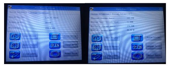
System settings, in the system settings, you can view the current system information, including the current application software version number, version type, and the IP address of the machine (if no Ethernet shows no support); can adjust the backlight brightness through a scroll bar; in calibration, the touch screen can be calibrated; IP The address can set the IP of the Ethernet HMI.
