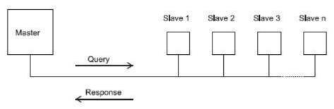
In the MODBUS Protocol the master can address individual slaves, or, using a special "Broadcast" address, can initiate a broadcast message to all slaves. The Brasiltec Digital meter do not support the broadcast address.
