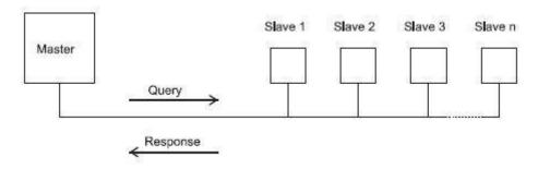
In the MODBUS Protocol the master can address individual slaves, or, using a special "Broadcast" address, can initiate a broadcast message to all slaves. The Brasiltec Digital meter do not support the broadcast address.
